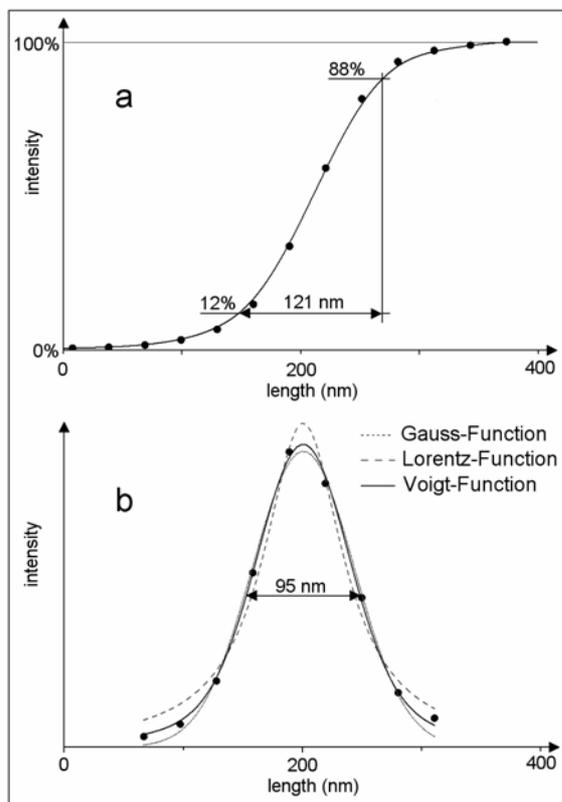
Fig. 3: Line profiles through different parts of the ToF-SIMS Al<sup>+</sup> image of Fig. 2.
