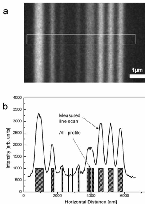
Fig. 4: a) ESCA Al 2p image of BAM-L002 taken at BESSY's UE52 SGM beamline at 150 eV excitation energy and 100 eV spectrometer analyser pass energy providing a Ag 3d<sub>5/2</sub> FWHM of 0.6 eV. b) The Al 2p line scan is constructed from the image data in the box inserted into Fig. 4a. The ideal Al profile to be expected from the BAM-L002 layout is inserted into Fig. 4b.
