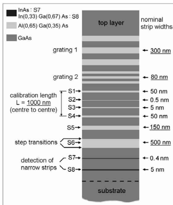
Fig. 1: Scheme of the strip patterns at the surface of BAM-L002. The underlined numbers are nominal values and the respective certified values are given in Tab. 1.
